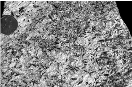
Schist (shiny with visible crystals of mica and other minerals)
